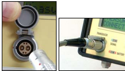
Fig. 7.1: Connection of the transducer
